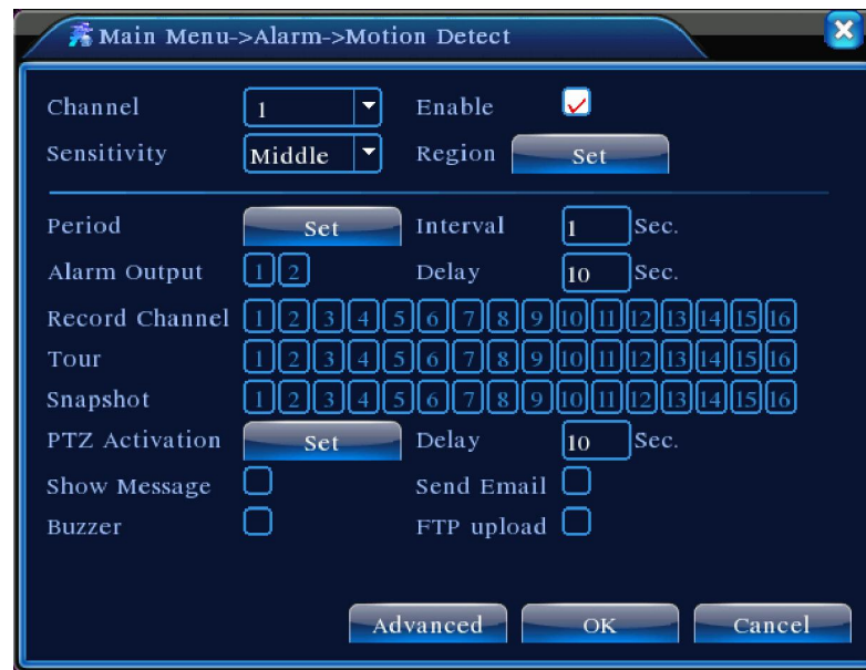
Picture 4.4 Hybrid mode(4+2) Motion Detect
