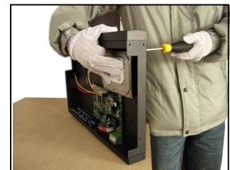
③fix the screw of hard disk
