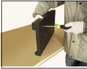
④fix the screw of hard disk
