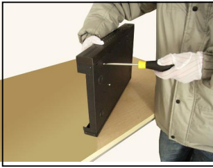
④fix the screw of hard disk
