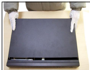
②disassemble the cover
